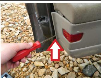
**STEP 7:** With the interior door trim panel removed from the door, disconnect the master power switch assembly.
