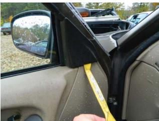
**STEP 2:** Remove the Phillips head screw attaching the interior door handle bezel assembly to the door.
