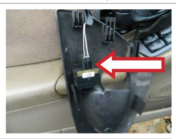
**STEP 4:** Using a pic or small flat-blade screwdriver remove the interior door trim panel attaching screw cover.
