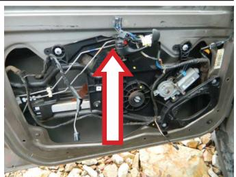
**STEP 13:** Remove the Phillips head screw that holds the interior door handle assembly onto the door.
