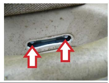
**STEP 11:** Install the interior door trim panel attaching screw cover.
