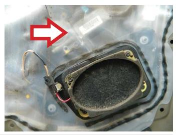
**STEP 12:** Disconnect the interior door handle latch rods from the interior door handle.
