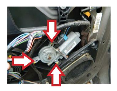
**STEP 3:** Install the window regulator assembly onto the door.
