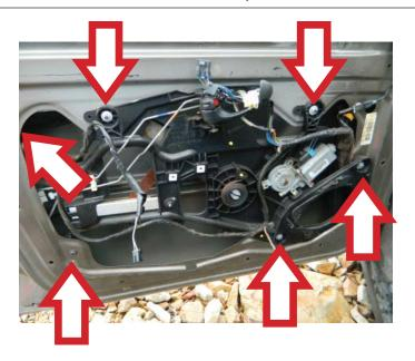
**STEP 4:** Temporarily install the master power switch assembly to raise or lower the window regulator for the door glass attaching points.
