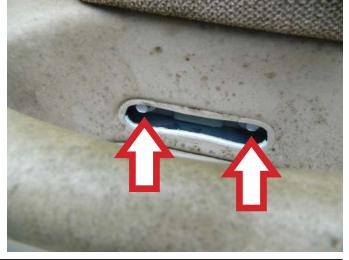
**STEP 6:** Using a trim panel removal tool, remove the interior door trim panel. **NOTE:** You may want to use a plastic trim panel tool to prevent scratching the painted surface.
