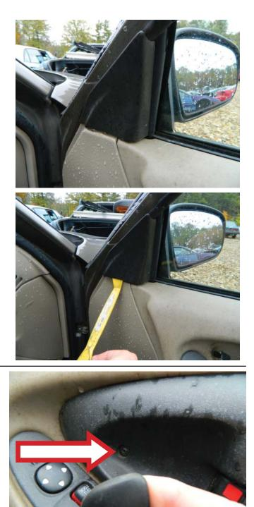
**STEP 2:** Remove the Phillips head screw attaching the interior door handle bezel assembly to the door.
