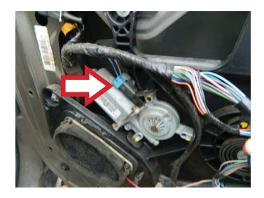
**STEP 15:** Remove the window regulator assembly attaching screws.
