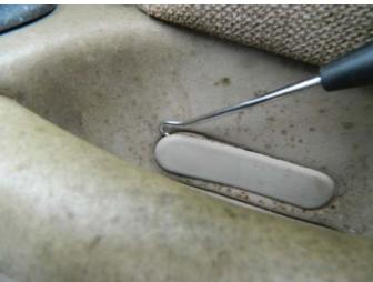
**STEP 11:** Install the interior door trim panel attaching screw cover.
