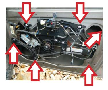
**STEP 4:** Temporarily install the master power switch assembly to raise or lower the window regulator for the door glass attaching points.
