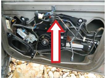
**STEP 12:** Disconnect the interior door handle latch rods from the interior door handle.
