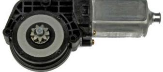
**STEP 1:** Attach the window lift motor with its three (3) mounting screws.
