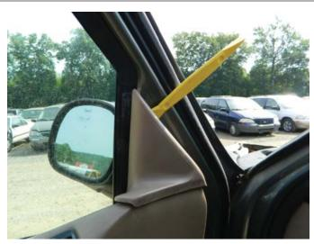
**STEP 3a:** Using a plastic trim panel removal tool, place the tool between the interior door trim panel and the rear view mirror bezel, and pry up in an upward motion.
