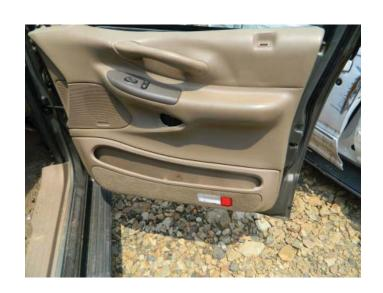
**STEP 2:** Disconnect the master power switch assembly.
