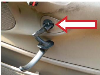
**STEP 10:** Remove the upper interior door trim retaining screw. The screw is located just above the interior door mechanism. The screw is somewhat obscure. Failure to remove this screw will not allow you to remove the door trim panel.
