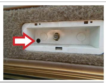
**STEP 16:** Install the door marker lamp lens assembly.
