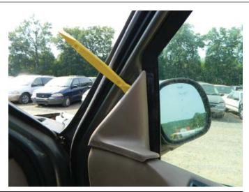
**STEP 3a:** Using a plastic trim removal tool, place the tool between the interior door trim panel and the rear view mirror bezel, and pry up in an upward motion.
