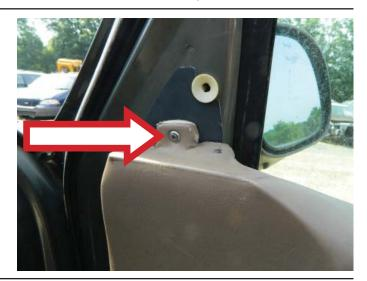
**STEP 14:** Install the upper interior door trim retaining screw.
