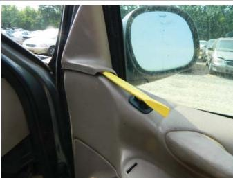
**STEP 4:** Remove the rear view mirror bezel assembly.
