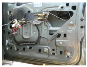
**STEP 15:** Disconnect the window lift motor connector.
