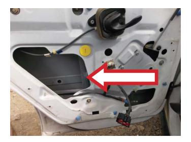
**STEP 13:** Remove the window regulator through the main access hole.
