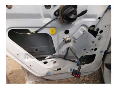
**STEP 7:** Install the water vapor barrier.
