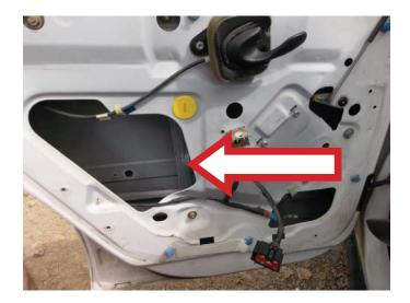
**STEP 1a:** Install the window regulator through the main access hole.
