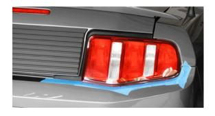
4. To carefully remove your stock lights, open your tailgate or trunk lid to access the back panel of your tail lights. Unscrew your worn out tail lamps from the front with the help of a Phillips screwdriver or undo of the bolts is released, your old lights may fall instantly. For this reason, it is better to lightly keep the lights in place with your free hand while you unscrew or unbolt them.
