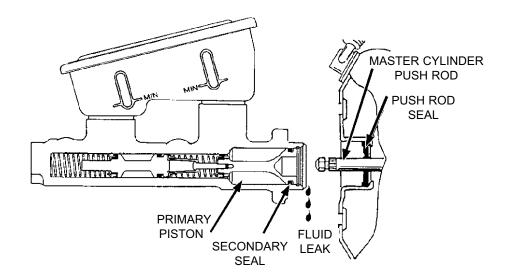
Note: When replacing brake components, always flush entire brake system with approved brake fluid from a sealed container.
