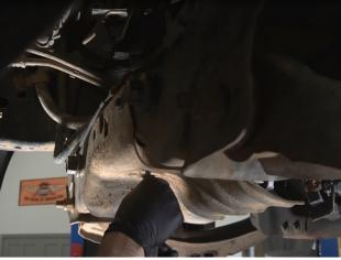
**STEP 8:** Tighten the jam nuts on the tie rod ends.
