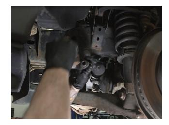
**STEP 5:** Reconnect the steering shaft to the rack and tighten the bolt to factory specs.
