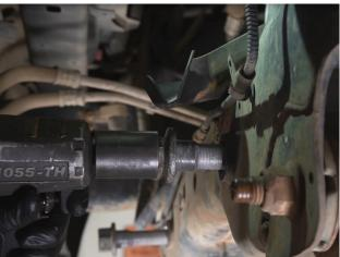
**STEP 12:** Work the steering shaft free from the rack, and carefully pull the original steering rack out of the vehicle.
