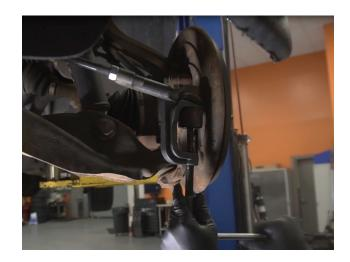
**STEP 10:** Remove the tie rod ends from the steering rack, if you're reusing them. **NOTE:** It may help to count and record how many turns are required, to speed up initial alignment when installing them on the new rack.
