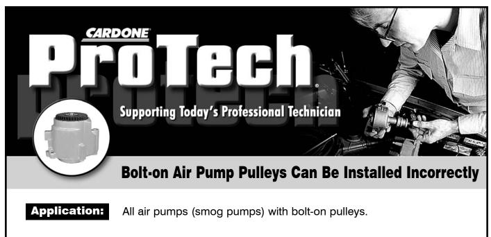
**Problem:** The original pulley rubs on the housing of the replacement unit, or the belt does not track correctly.
