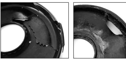
Typical vacuum booster diaphragm failure due to gas or gasoline fumes
