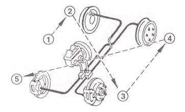
When replacing brake components, always flush entire brake system with approved brake fluid from a sealed container.
