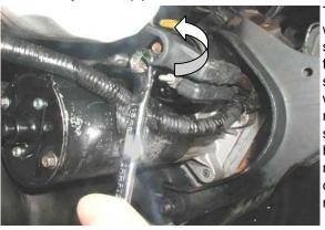
This cable will be secured to the starter's solenoid with a large nut. Some starters may have a rubber boot covering the nut.
