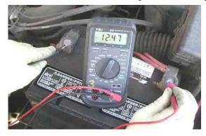
1) Check to make sure the battery is charged to 12.4-12.6 volts. If it is not, check the battery fluid level (if it is low, add distilled water to bring the level up to the fill line) and charge the battery now 2) Now turn on the headlights if the voltage drops below 12.1v, the battery may be bad.
