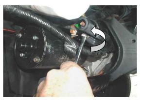
This lead may be attached to the starter with a spade connector, plug, nut, or screw.
