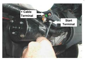
**NOTE:** DO NOT OVER TIGHTEN the positive (+) battery connection. This may break the solenoid cap damaging your new starter.
