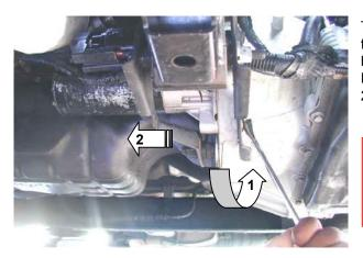
The mounting bolts may be accessible from either the starter side or the bell housing side (as shown in the photo). 1) Remove all mounting bolts and hardware 2) slide the starter out of the vehicle.
