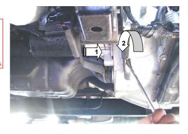
8 Install the electrical connections. Install the positive (+) cable and start terminal lead.
